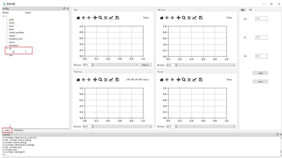
2. Directly after the modification, close the current window and reopen it, you can find that there is no driver board information in the upper computer as shown in the following figure, because the driver board id has been modified to 2.
