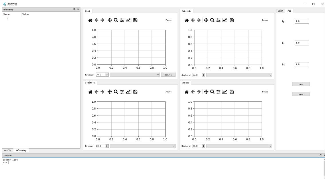
3. Next, we close both windows of the host computer, re-open the host computer, the host computer will automatically recognize the changed ID, click "**Open Tview**", in the command line of the host computer, enter the save command **conf write** to save the ID, the feedback is **OK** that is, the ID is successfully modified, as shown in the figure below.
